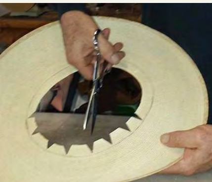
Step 3: Cut triangles out, to the edge of the line, to make tabs.
